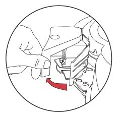
Figure 3. Separating the Printer Cover from the Left Access Door
