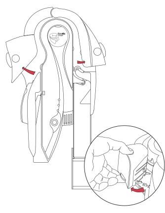
Figure 2. Opening the Left and Right Access Doors
